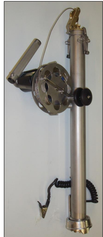
Winder MK 2, with Depth Counter & UTI type coupling
