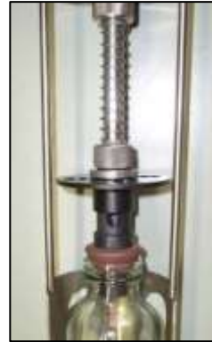
Inlet valve set to maximum opening (for viscous oils)
