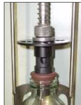
All-level Sampling: Inlet valve set to maximum opening (for viscous oils)
