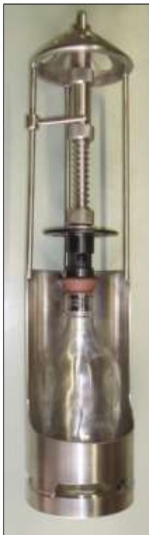
All-level sampler set-up
