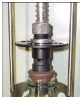
All-level Sampling: Inlet valve set to minimum opening (for light products)
